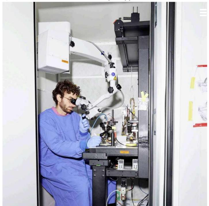
Fadhel El May and his colleagues insert the implants into the gerbils in a so-called "soundproof chamber." The cabins are soundproof to ensure that no disturbing noises distort the results during the acoustic experiments.
